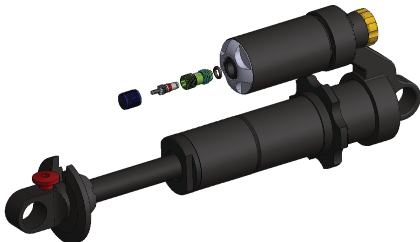
Figure 9. Marzocchi Bomber CR with Shockcraft Faux IFP Valve Stem Kit.
