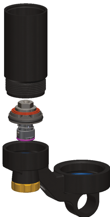
Figure 6. Install of base valve in piggyback.
